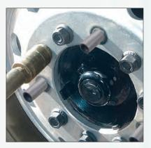
Our new threadless design allows the installer to quickly and easily center the wheels to the hub. And our tapered design makes it easy to mount the wheel over the hub.
