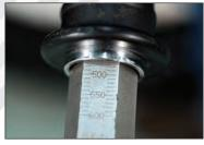
Hub-Pilot Wheel: 450-500 ft/lbs. oiled | Stud-Pilot Wheel: 450-500 ft/lbs. dry | Demountable Rim: 200-260 ft/lbs. dry
