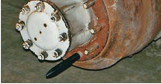
The O-Line-Er Wheel Stud Alignment Tool makes it easy to line up wheel studs with holes in rim for easy installation.
