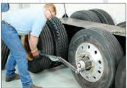
stands for torque the fasteners to specification
