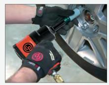
The 1/2" Super Duty Air Impact Wrench-Tire Tool in use.
