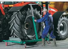
The Wheel Dolly for Agricultural and Earth Moving Machinery makes possible easy and safe mounting, demounting and handling of large wheels.
