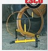
The Ring Master O-Ring and Lock Ring Installer in use.
